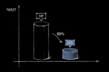
LED-based SunSphere technology from KBL reduces power consumption by up to 80% compared to conventional highpressure systems using UV lamps.
